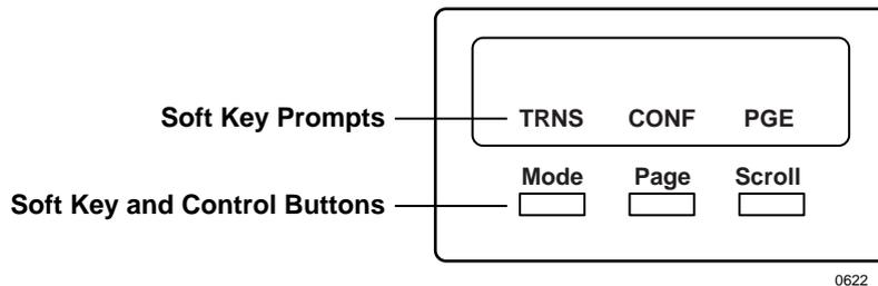
Figure 3 LCD Buttons (with sample Soft Keys)
